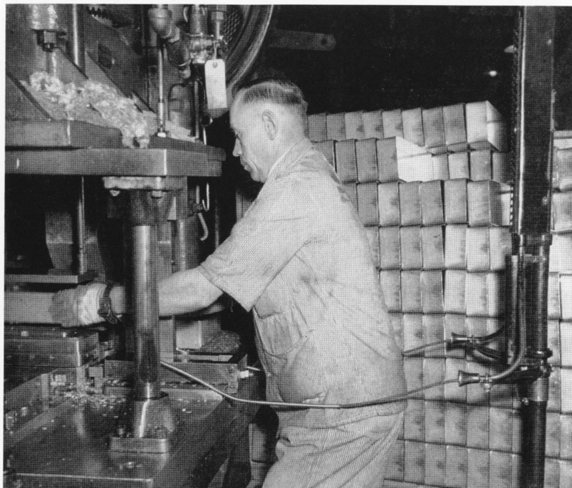
Walter Osowski of the Blanking Room demonstrates the correct method of operating a clipping machine with the Posson Safety Device (wrist straps). This machine took two fingers and part of a third from one operator, who has not yet fully recovered from the injury. He was not wearing the straps.
